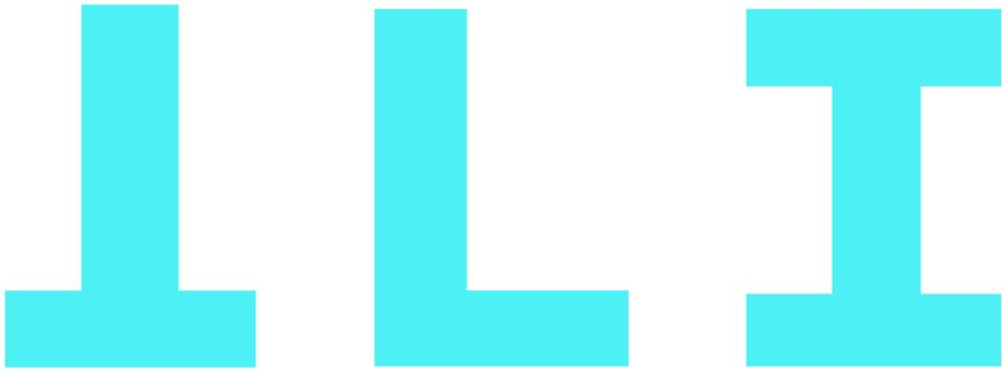
Fig. 3 Cross-sectional shapes of helideck member group
