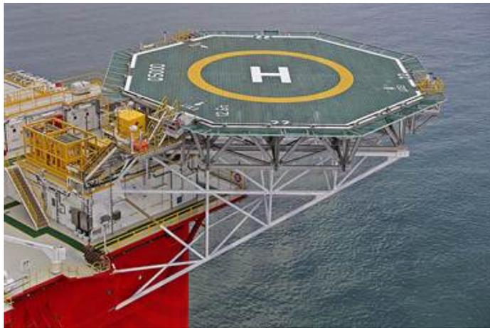
Fig. 1 Cantilever-type helideck
