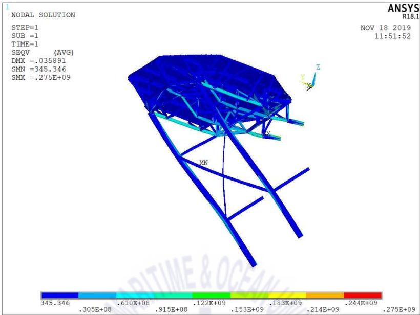
Fig. 22 Equivalent stress distribution for OPT-4 model
