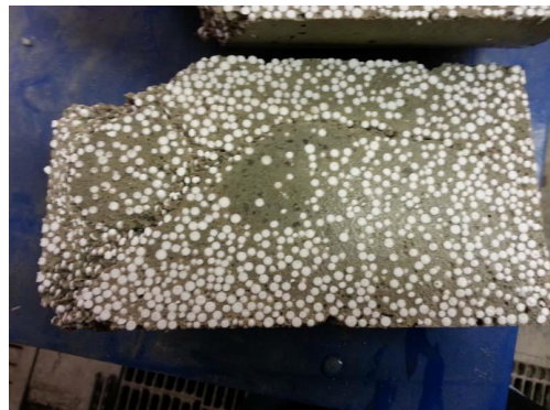
Fig. 2-11 Crushable Concrete (Doyle et al. 2016)
