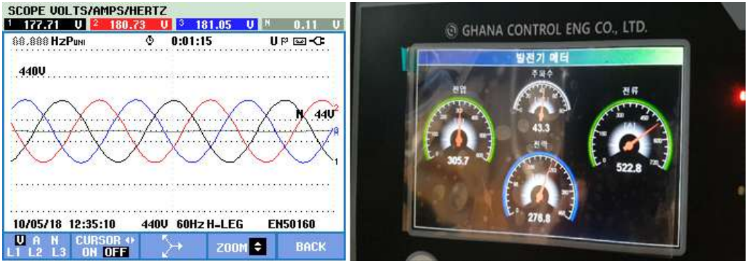
Fig 5.19 Generator output voltage, current, frequency(1300rpm)
