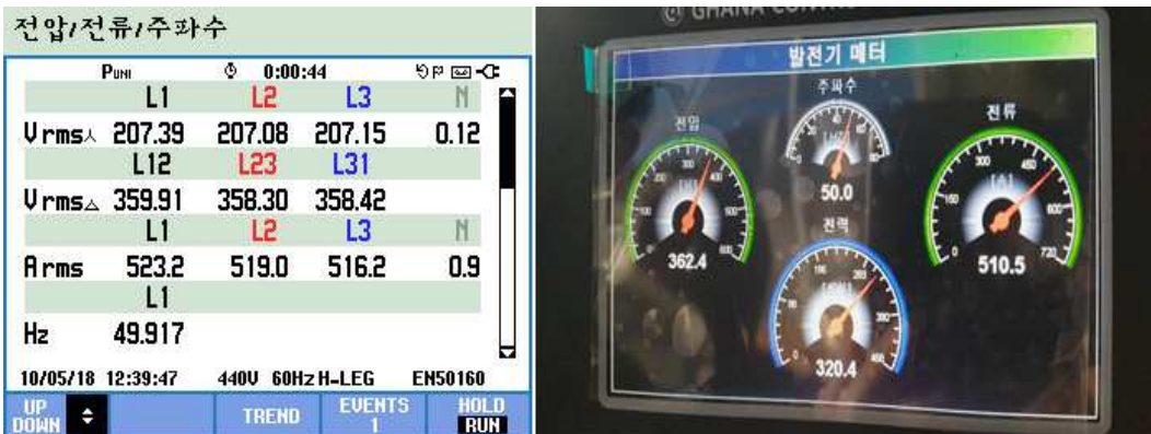
Fig 5.20 Generator output voltage, current, frequency(1500rpm)
