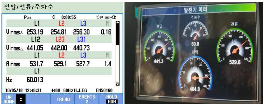
Fig 5.22 Generator output voltage, current, frequency(1800rpm)
