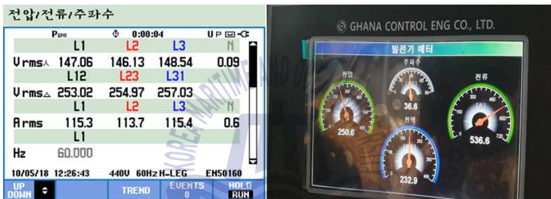
Fig 5.18 Generator output voltage, current, frequency(1100[rpm])
