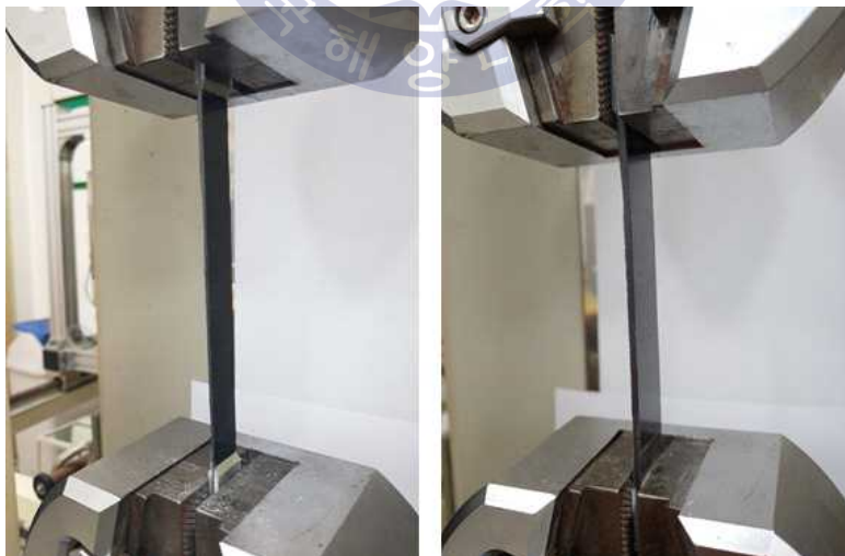
Fig. 16 Tensile test (longitudinal and transverse direction)
