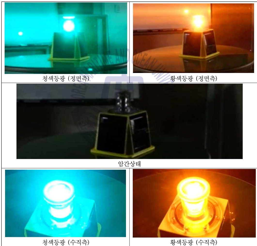
Fig. 70 Flashing test of Lantern
