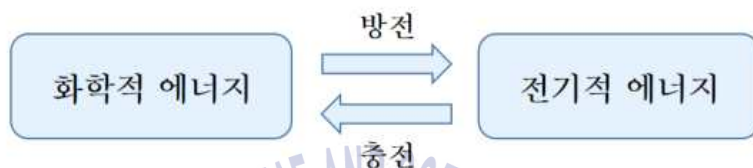
Fig. 29 Energy Exchange of Battery
