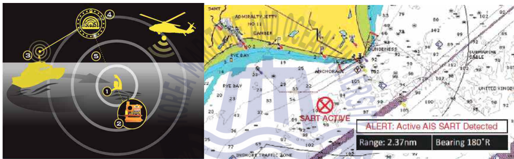
Fig. 26 MOB utilization, Electronic Chart Display
