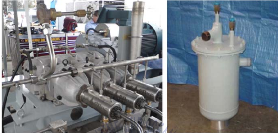
Figure 2.5 HP pump and HP vaporizer [49]
