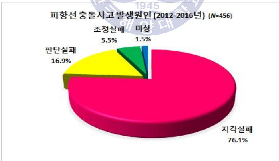
Fig. 19 Causes of collision accidents(give-way vessel)
