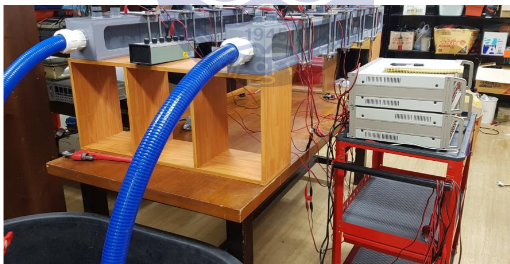
Fig. 3.5 Picture of Cathodic protection test
