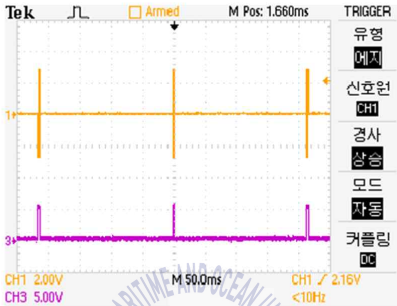
Fig. 5.18 RS-485 Communication to transmit pressure data waveform
