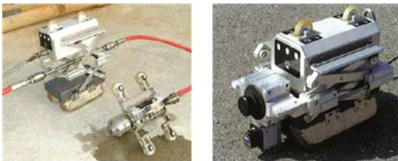
Fig. 1.5 Configuration of the water-jet cleaning robot for WARECO
