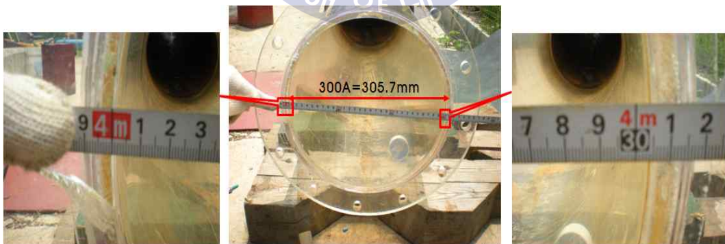
Fig. 5.7 Dimension of the observation pipe (300A)
