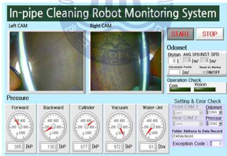
Fig. 4.14 GUI-based monitoring program
