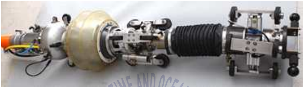
Fig. 2.18 Prototype of the pipe cleaning robot
