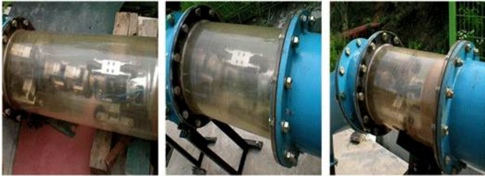
Fig. 5.8 Observation pipes in the test bench
