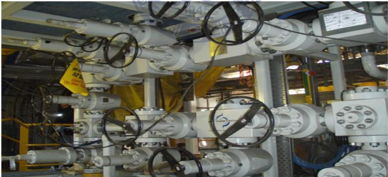
**Fig. 3.1** Choke & Kill manifold
