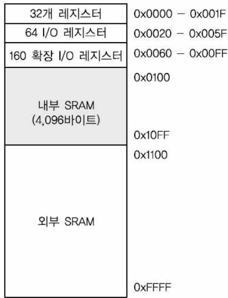
Fig. 14 Data area memory map of ATmega128
