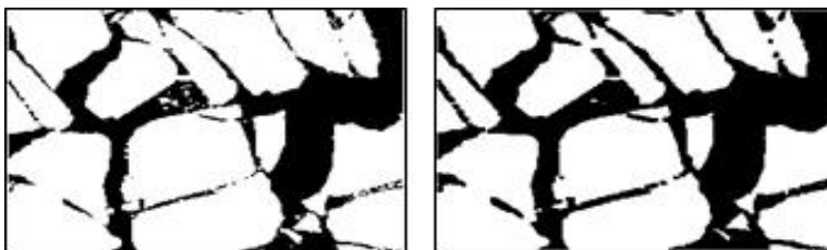
Fig. 51 Binary image(left) and morphology erode image(right)
