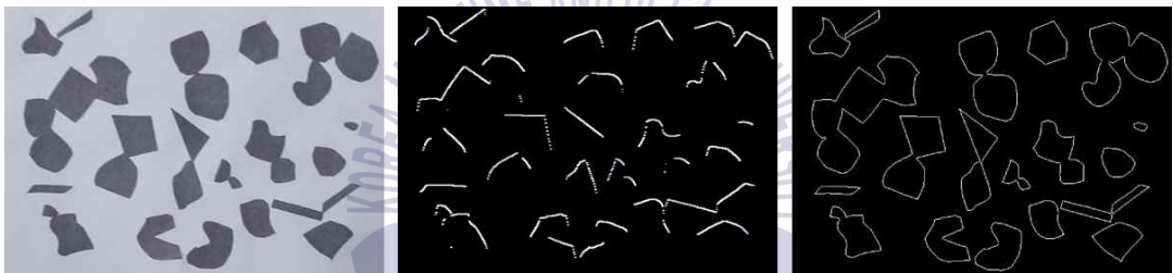
Fig. 50 Primary(mid) and secondary(right) derivative edge of original image(right)
