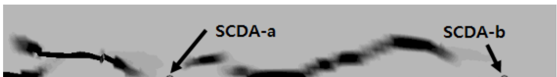
(d) 2m (Second crack path between SCDA-a and SCDA-b)
