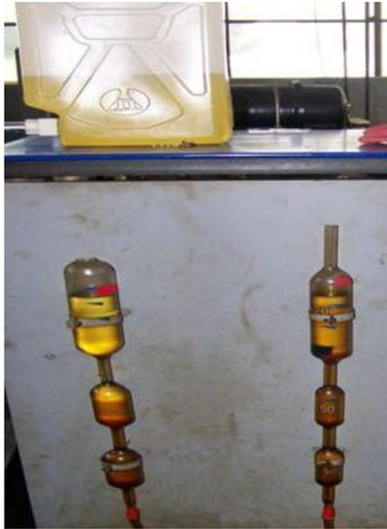
Fig. 11 The buret for fuel consumption measurement
