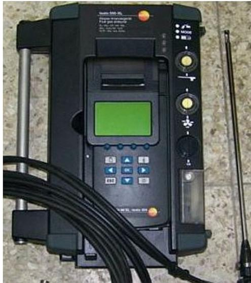
Fig. 13 Tester for emission ingredient
