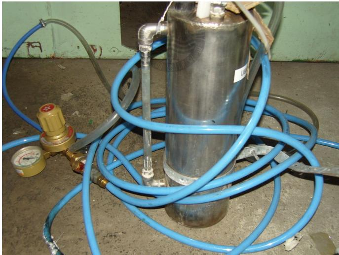
Fig. 15 Photo of 2000ml/min type hydrogen generator
