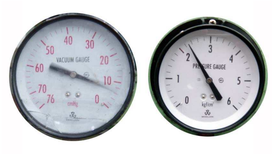
Fig. 3.6 Suction / Discharge gauge
