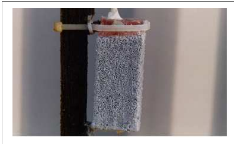
(b) Al anode specimen after 10 days (with rusted steel pile)
