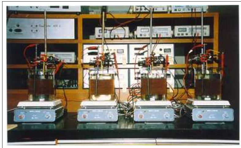
(b) No stirring & stirring, rusted Fe specimen
