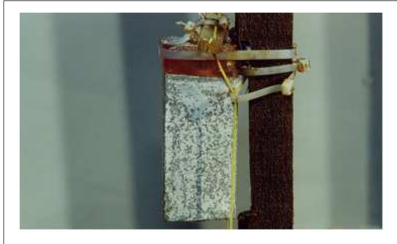
(a) Al anode specimen after 10 days (with steel pile)
