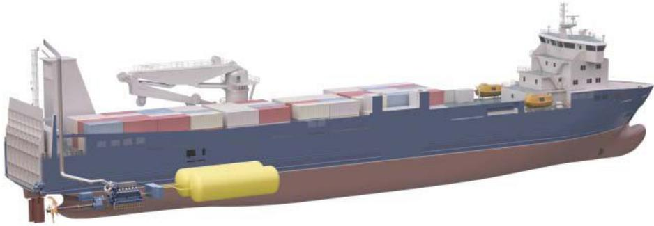
LNG tanks and propulsion machinery are situated low in the vessel to enable easy vehicle access via the ramp and maximize the available cargo space. The tanks may also be situated on open deck.
