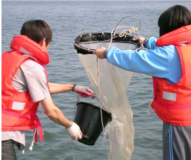
Fig. 4. Picture of zooplankton sampling with zooplankton net(mesh size 330\mu\text{m} ).
