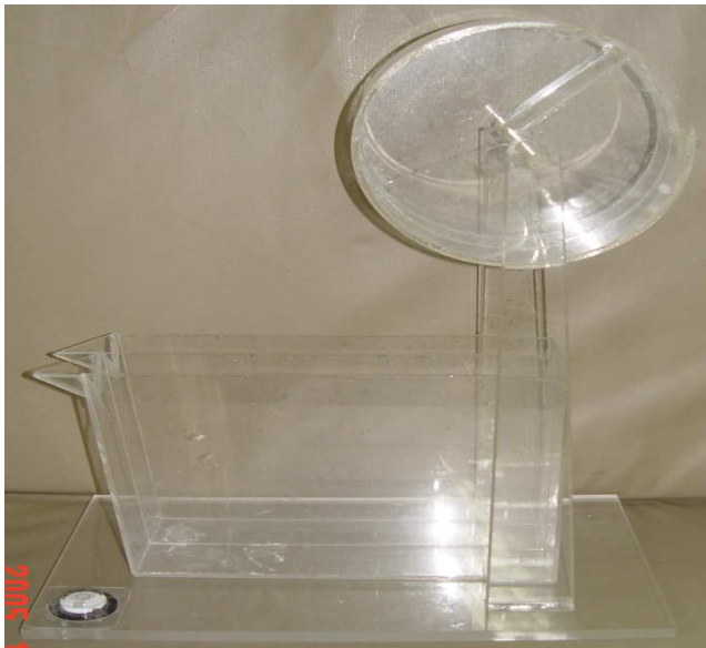
Fig. 5. Picture of modified Folsom splitter made in our own lab for separating zooplankton samples.
