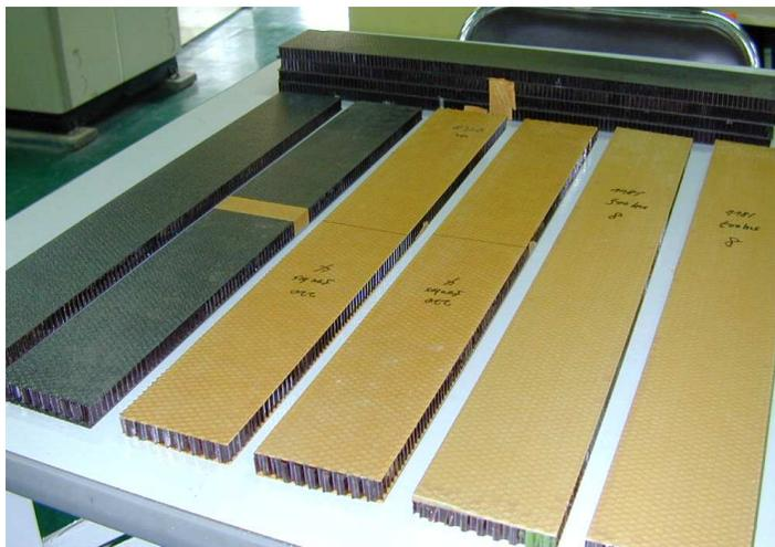
(c) Long beam flexural specimen
