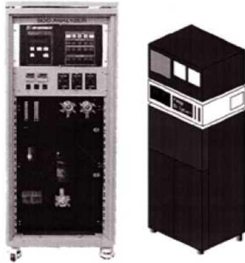
Fig 2.4 Photograph of BOD monitoring system which use a microbial fuel cell
