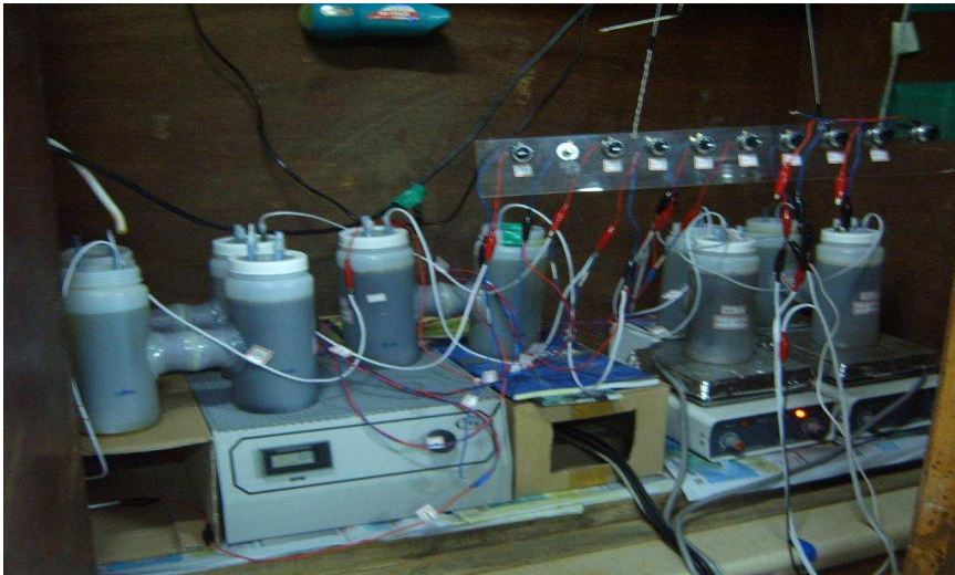
Fig.3.1 Photograph of dual chamber batch MFC system
