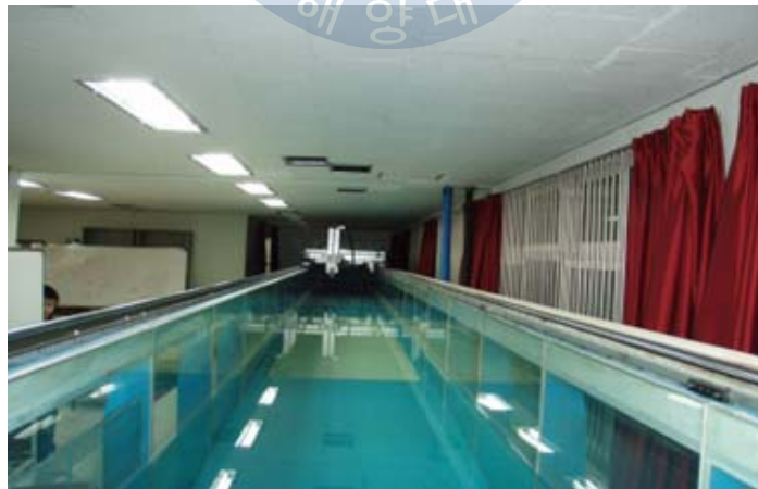
Fig. 3.1 Two-dimensional ocean engineering basin
