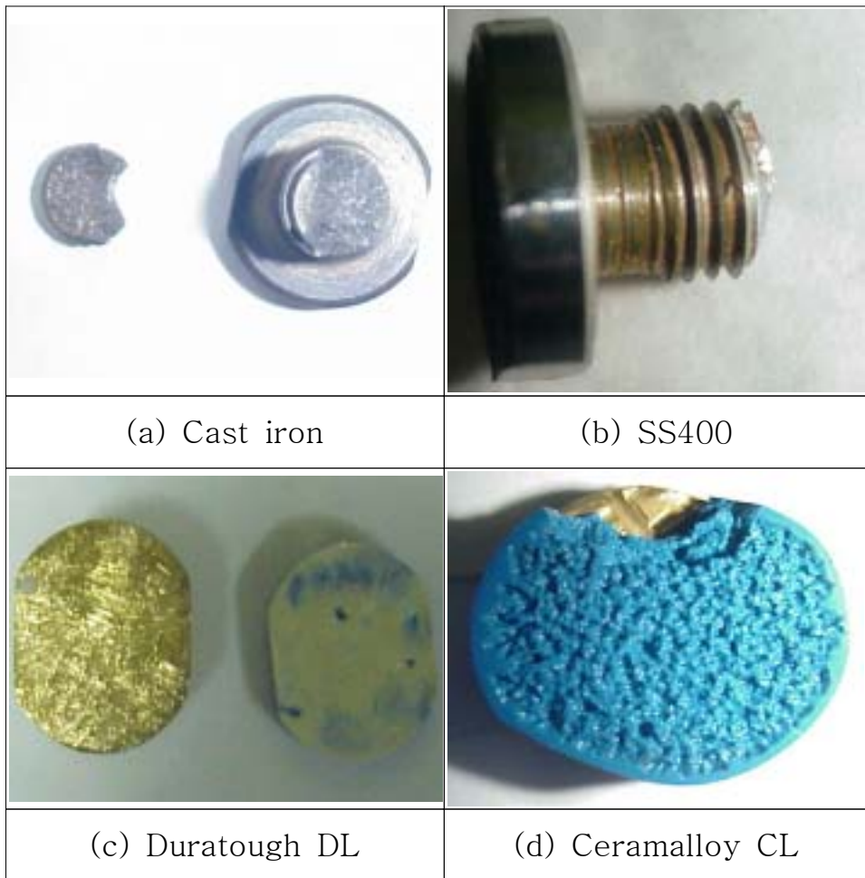
Photo.4 Fractured surface in standard test.
