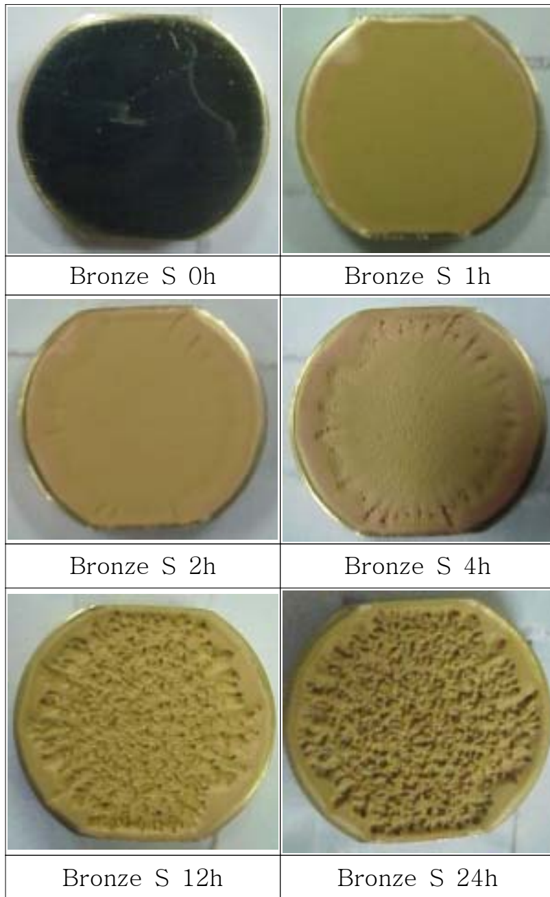
Photo.8 Successive observation of damaged surface according to test time(0, 1, 2, 4, 12, 24 hour) in sea-water for Bronze.
