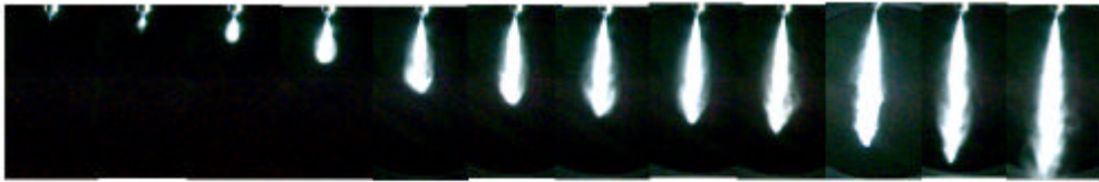
(a) Rail pressure 10MPa - Surround pressure 0MPa
