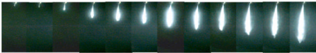
(b) Rail pressure 10MPa - Surround pressure 0.3MPa
