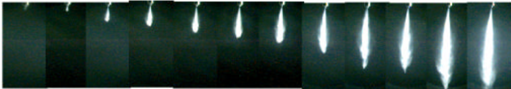
(a) Rail pressure 10MPa - Surround pressure 0.0MPa
