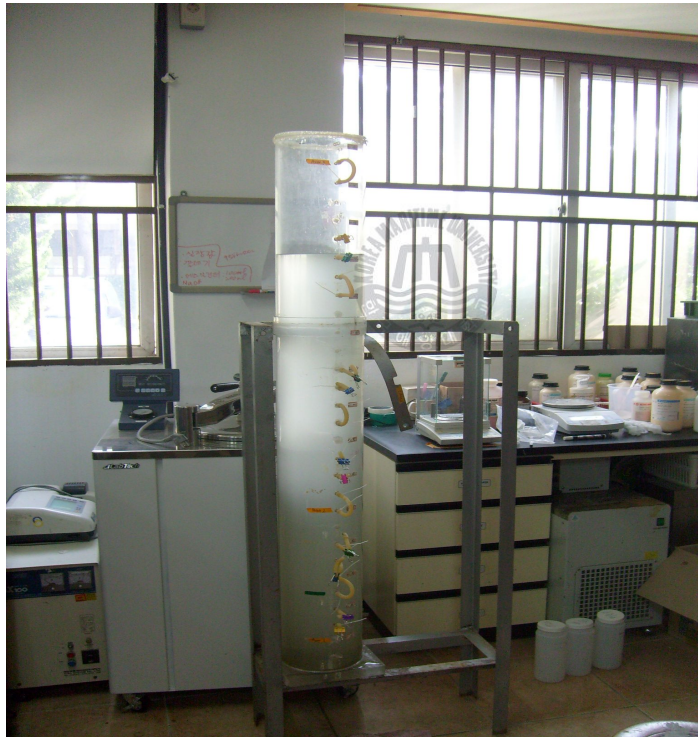
Fig 3.3 Sedimentation tests of red tide remediation materials
