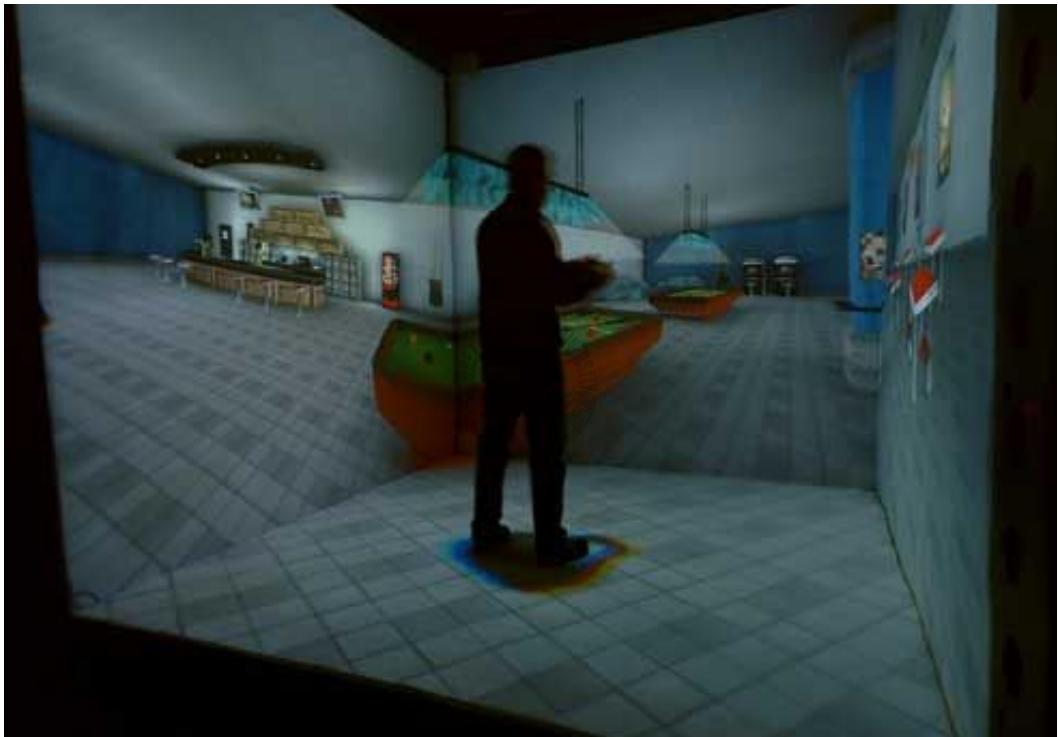
Fig. 1 Three Dimensional Cube Stereo Visualization Cluster System
