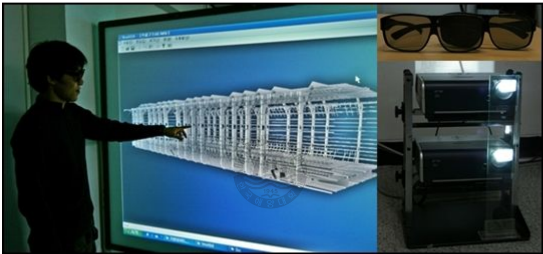
Fig. 8 Passive Stereoscopia Display System
